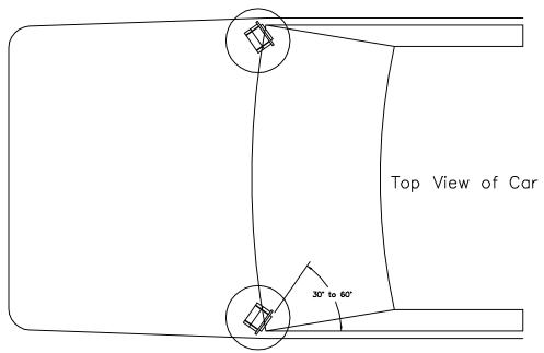
Mount the hinge so that the edge toward the outside of the car is 30 to 60 degrees forward from the inside edge. The top face of the hinge should be about flush with the upper back edge of the fender.
