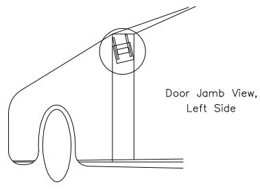
Mount the hinge so that the top edge is rotated as much as possible toward the outside of the car and the bottom end of the hinge is rotated as much as possible toward the interior.
